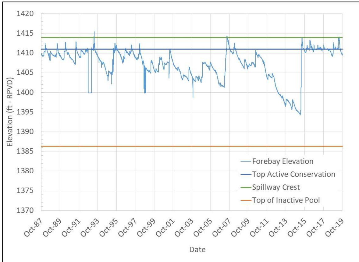
Figure 10. Historic Tom Steed Reservoir forebay water surface elevations (RPVD). Data web source: https://www.usbr.gov/gp/hydromet/archive.html
