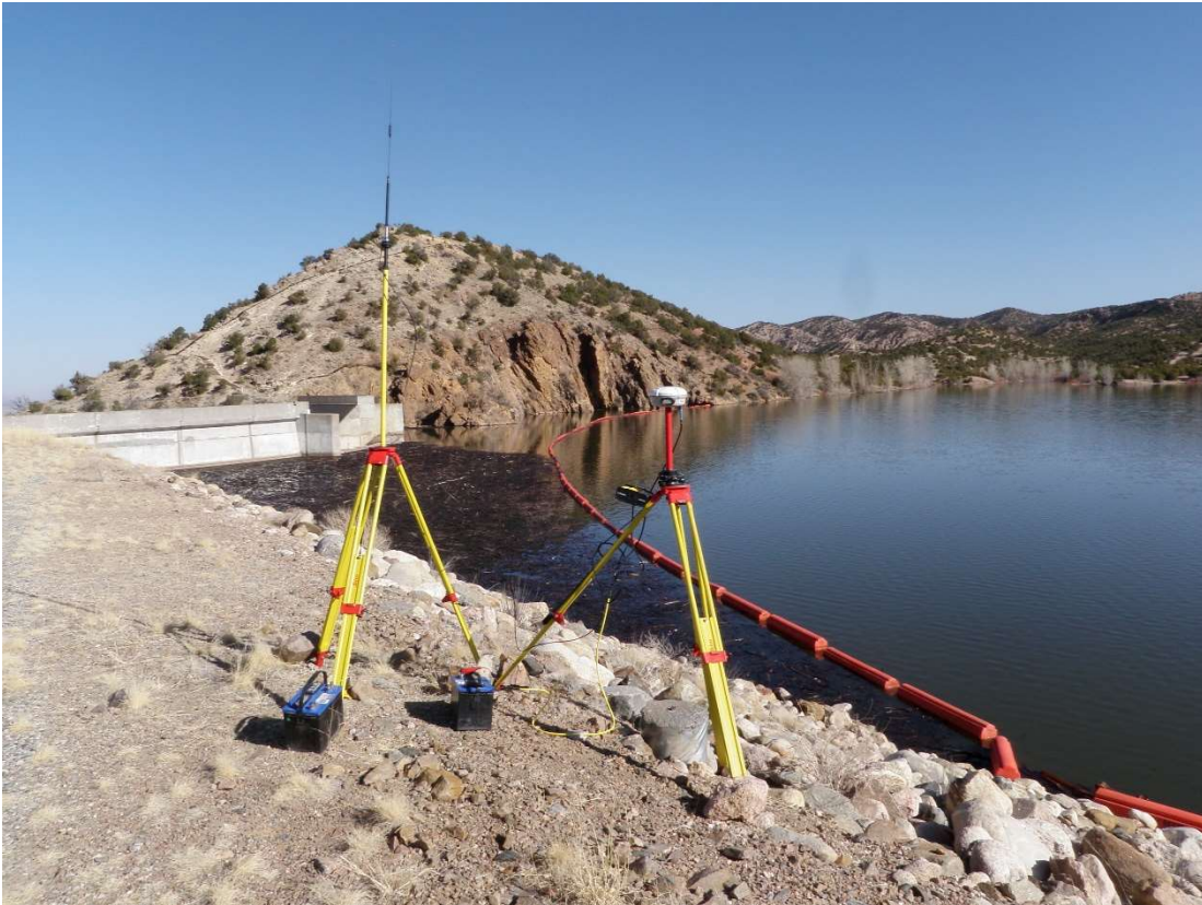
Figure A-2. The RTK-GPS base station set-up used during the Nambe Reservoir survey in New Mexico is typical of the set up used at Tom Steed Reservoir.
