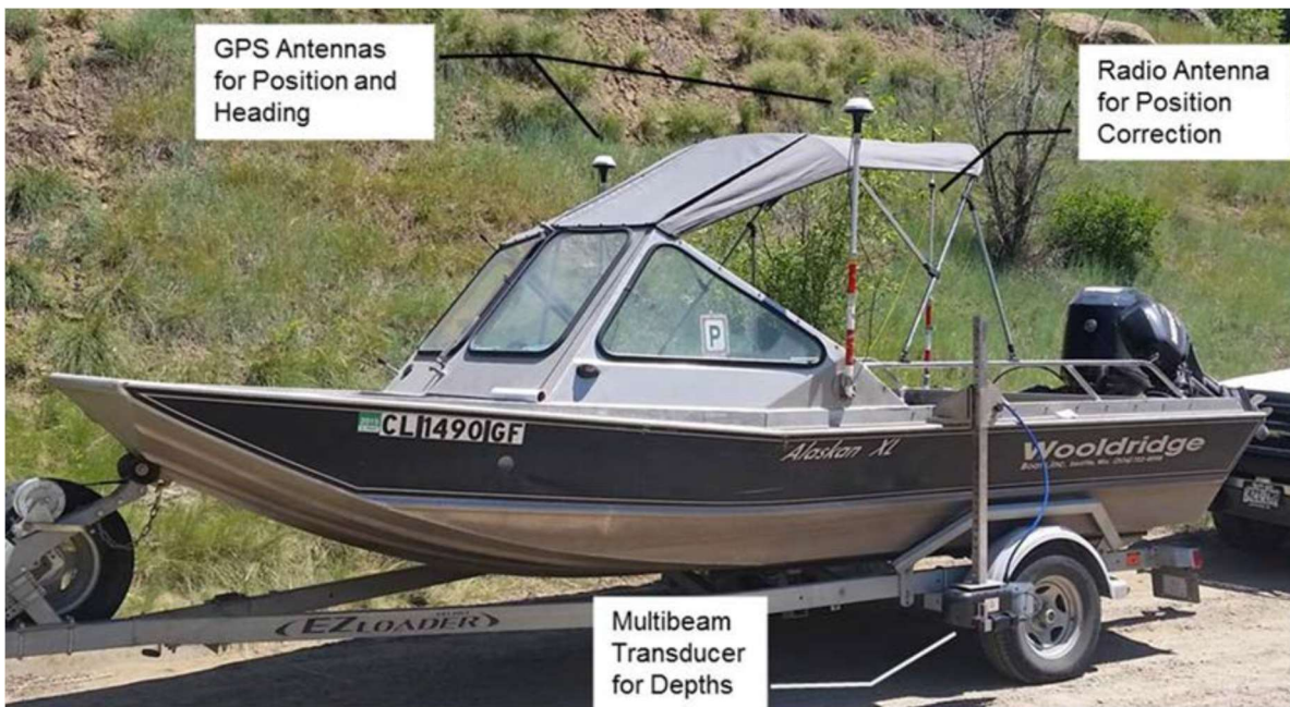
Figure A-1. Wooldridge boat with RTK-GPS and multibeam depth sounder system.
